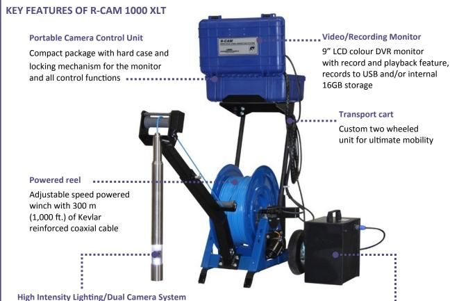
50 super bright, water-clear LEDs with five stages of adjustable lighting which allows high resolution videos in wells up to 30.5cm in diameter.
